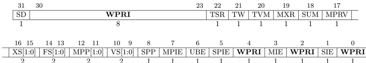
Figure 3.6: Machine-mode status register (`mstatus`) for RV32.
