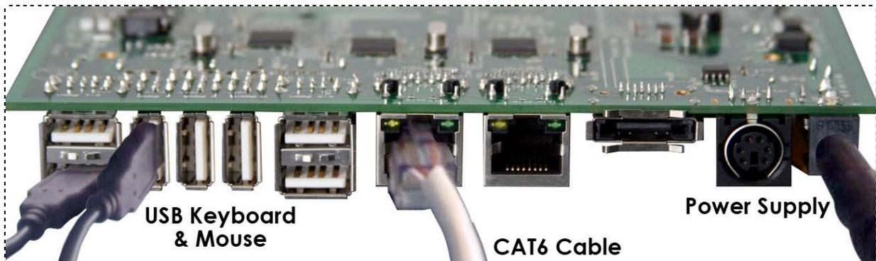
Figure 4 OpenRD-Client - USB, GbE0, and Power Supply
